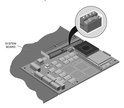
If the jumpers and switch are not as shown above, reconfigure the socket by moving the jumpers and switch to the correct positions.
