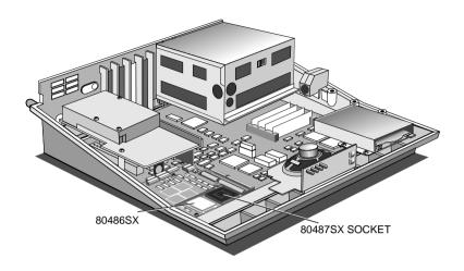
From the illustration above, you will be able to identify the 80487SX socket. If the socket is unoccupied, and an 80486SX is soldered to the CPU module as shown, you can install the 80487SX as described in *Installing the 80487SX*.
