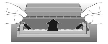
8. If the SIMM is properly located the SIMM should remain in position held by the securing clips, and with a small plastic lug through the holes on either side of the SIMM.
