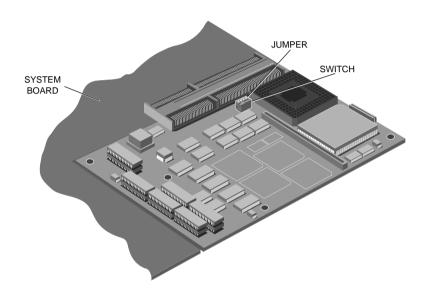
If the socket is configured for an 80487SX two jumpers will be fitted and the switch will be away from the socket, as shown in the following illustration.
