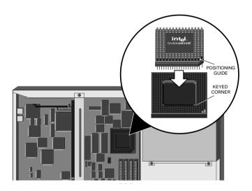
Carefully position the upgrade processor above the socket with the positioning guide on the processor over the keyed corner of the socket.
