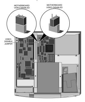
4. Remove the jumper clip from the two pin connector and replace it on only one of the connector posts as shown above.
