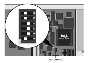
The switches numbered 2 and 3 are used to select the system clock speed. Switches 4 and 5 are used to configure the upgrade socket.
