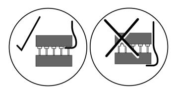
Be careful to ensure that the prongs do not go between the motherboard and the socket.
