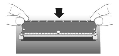
3. Lower the SIMM into the socket, and ensure that the SIMM is properly located in the connector.
