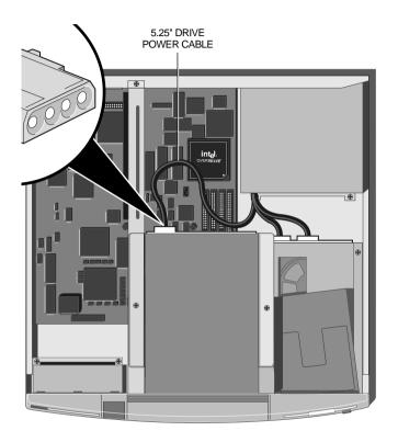
19. The drive has now been installed and connected to a power cable. You must now connect it to a signal cable. Instructions on connecting each of the types of drive to a signal cable is given under the appropriate heading overleaf.
