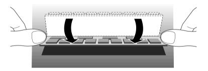
If the SIMM is properly located the SIMM should remain in position held by the securing clips, and with a small plastic lug through the holes on either side of the SIMM.
