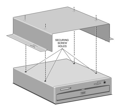
12. Line up the holes in the underside of the drive with those in the base of the drive bay.
