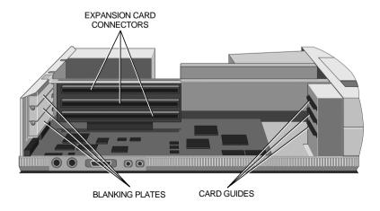
At the rear of the area are three metal blanking plates, one for each expansion card slot. These plates cover slots in the rear of the system unit which will be used by expansion cards.
