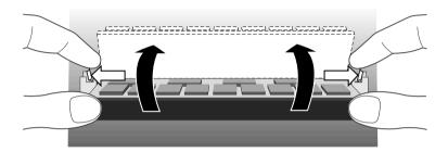
When the SIMM has rotated through 20°, taking care to avoid touching any of the components on the SIMM, grip the top corners of the SIMM between thumb and first finger and carefully pull the SIMM out of the socket.
