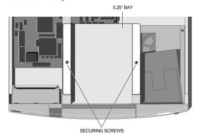
4. If there is a drive fitted in the 5.25" bay disconnect the power and signal cables from the rear of the drive.
